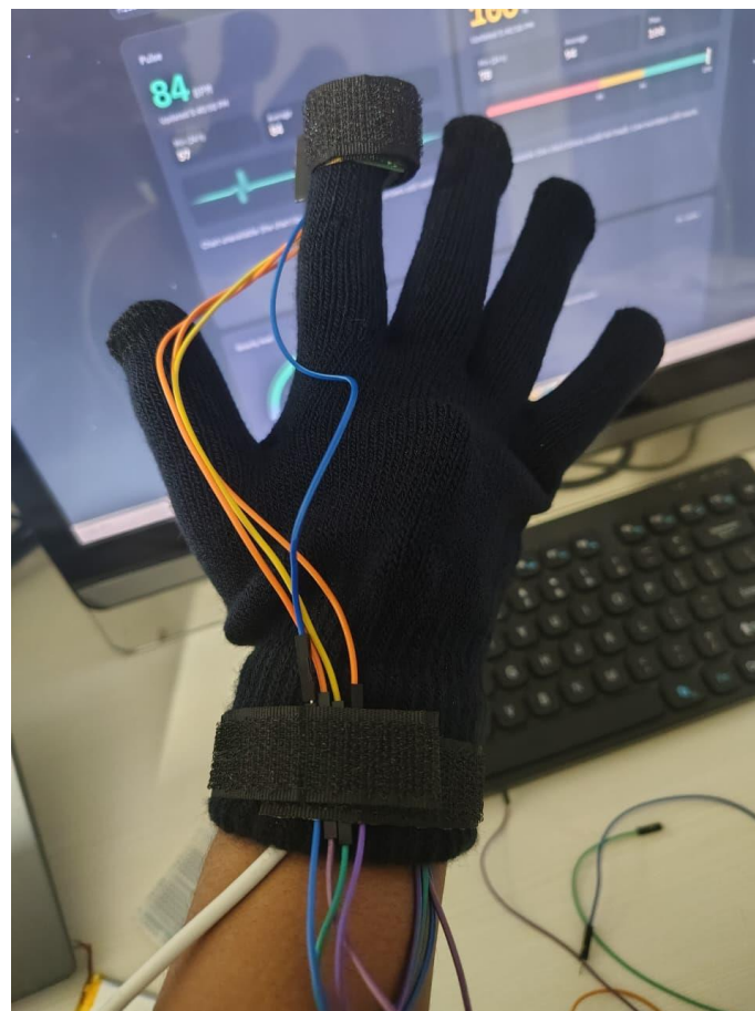
Fig. 4. Assembled glove-mounted AstroPulse prototype with fingertip MAX30102 sensor, routed jumper wires and Velcro wrist support.
